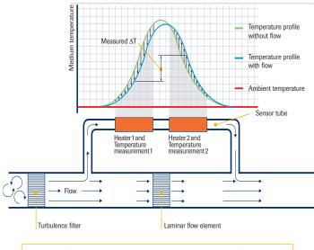
$\Delta T = k.C. \emptyset_m \Delta T = T2-T1$  in Kelvin  $C_n = \text{specific heat } \emptyset_m = \text{mass flow}$
